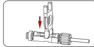
When uninstalling DC input connectors, insert removal tool into the bayonet as shown in Figure, press the tool down, and take out the connector.
