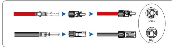
**WARNING** When taking out DC connectors, please ensure that PV Strings are disconnected; otherwise, a fire can occur.
