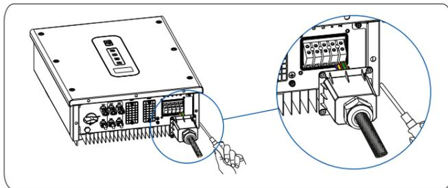
Step 6 Use a torque wrench to tighten cable gland with 5N·m
