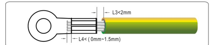
Step 3 Secure the PGND cable using the ground screw and tighten the screw to a torque of 1.2 N·m.
