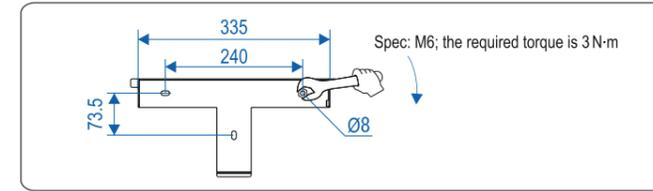
Step3 Mount the inverter on the rear panel and keep them aligned with each other.
