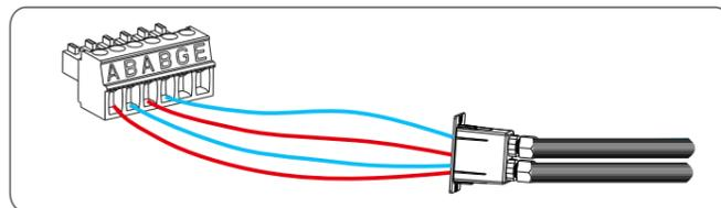
Step 5 Connect 6-pole male terminal to its female terminal. Lock the case to the inverter with two hexagonal screws and tighten the cable gland.
