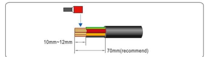
Step 2 Insert the exposed core wires into the crimp area of the supplied insulated end sleeve terminals and crimp them using specific tools.
