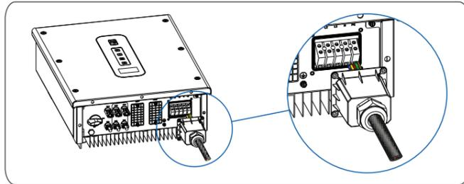
Step 4 Rout AC output cables to L1, L2, L3, N, and E on the AC terminal block respectively, and tighten them using screw driver to a torque of 1.5N·m.
