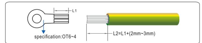
Step 2 Insert the exposed core wires into the crimp area of the OT terminal and crimp them using hydraulic pliers, and crimp them with hydraulic crimping pliers.
