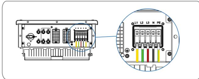
Step 5 Fasten the AC terminal cover by four hexagon screws supplied; tighten the screws to a torque of 0.8 N·m.
