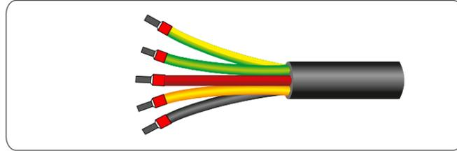
Step 3 Insert the prepared AC output cables through AC waterproof cover with reserved wire length for electrical connecting.
