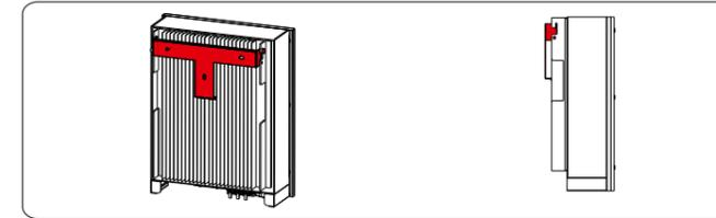
Step4 Tighten the retaining screw on the rear panel to fasten the inverter.
