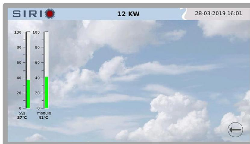
The temperature called SYS is the internal temperature of the machine.
