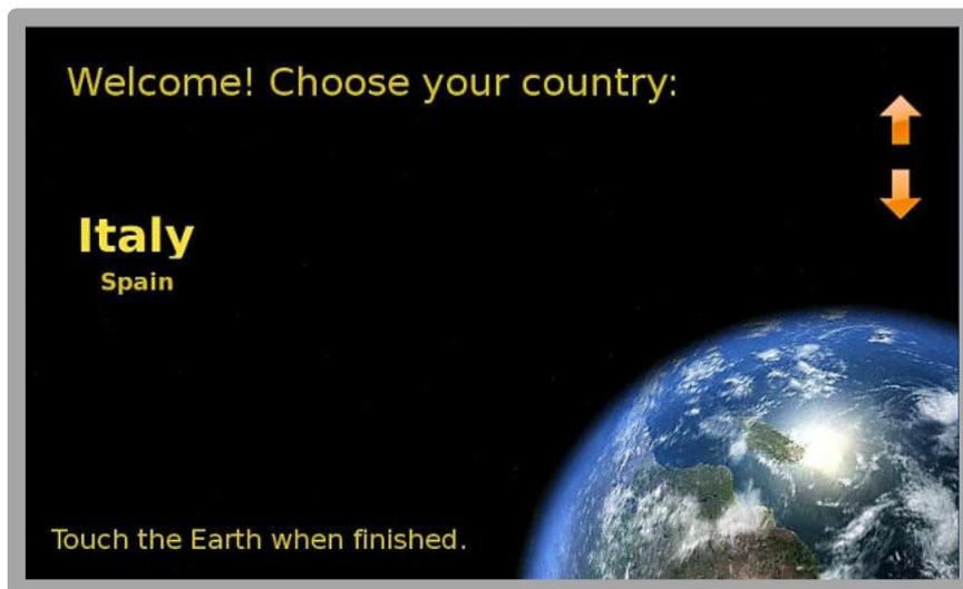
The user can scroll through the countries currently managed using the arrows on the right of the screen; after selecting the correct country, simply touch the earth image to proceed with the configuration:
